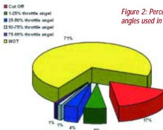
Figure 2: Percentage of the throttle angles used in a Le Mans race lap
