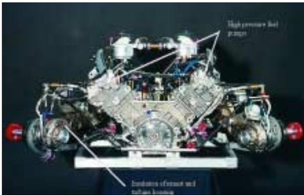
*Figure 7: Audi R8 with V8 FSI twin turbo engine*
