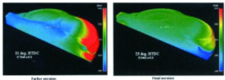
*Figure 6: The optimum interaction between the spray geometry and the tumble is the key to achieving optimum homogenisation. This figure shows two different examples.*
