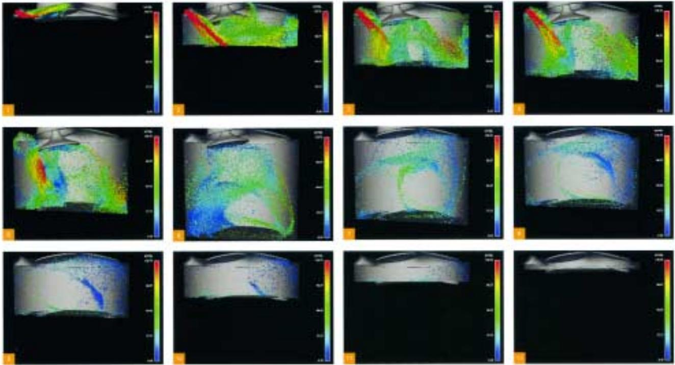
*Figure 5: The CFD calculation was carried out in order to gain information about the mixing process between the injected fuel and the air forced into the tumble motion.*
